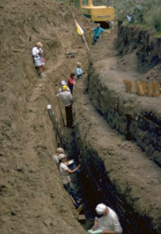
Figure 5. Trenches were dug at Morefield Reservoir to study sediment layers.
